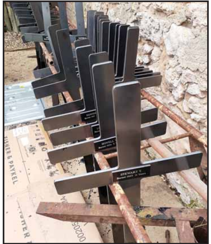
ABOVE: Crosses drying from being dipped with bitumen
